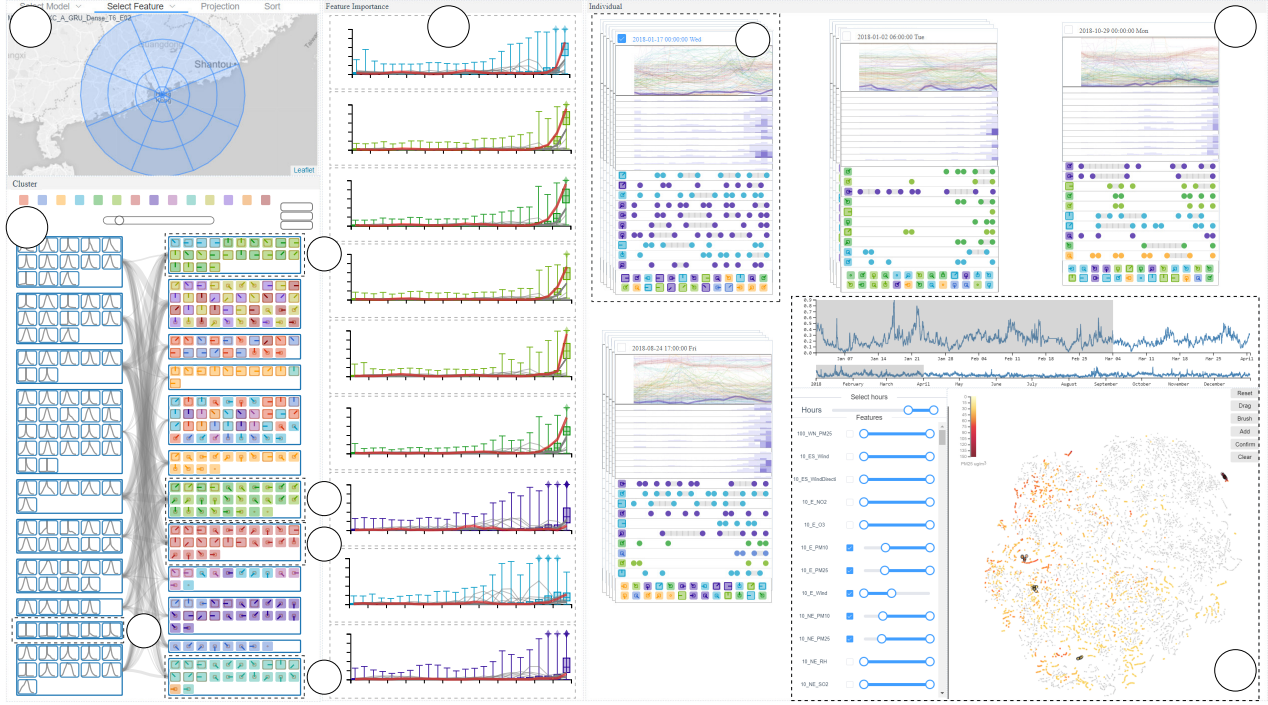
Figure 5: MultiRNNExplorer contains multiple coordinated views to support exploring and understanding RNNs' behaviors on multi-dimensional time-series data, especially on hidden unit response and feature importance. The Configuration Panel (B) allows users to select an RNN model and configure parameters. To reveal model mechanism, the Cluster View (A) summarizes the hidden unit clusters' response to feature clusters, and the Feature Importance View (C) summarizes the temporal importance of input features. The Projection View (E) displays a data overview, allowing users to select sequence instances of interest for further analysis. The selected instances will be shown in the Individual View (D).
