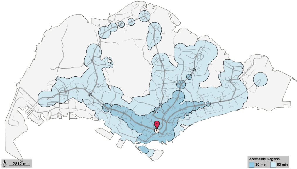
Figure 6.2: The isochrone map view presents spatial-reachability regions from 08:00 at origin A (red icon), which is station XX16/WW3 in the city center, by contour lines and areas over the geographical map. Dark blue and light blue indicate [0, 30] and (30, 60] minutes, respectively.
