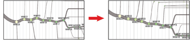
Fig. 8. Left: up-and-down wobbling. Right: we fix it by vertically shifting the nodes by node-based moving-window averaging.
