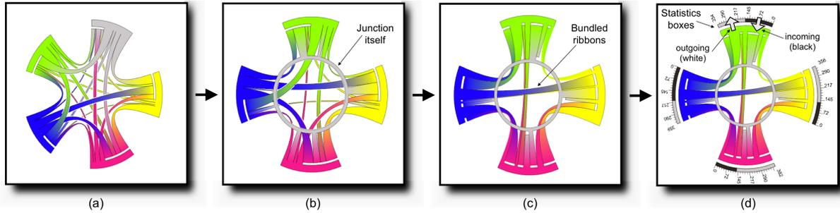
**Figure 5:** Developing the interchange circos diagram from the original circos figure: (a) the initial design in Figure 4; (b) use a grey-colored flyover ring (like a source/sink for the junction itself); (c) bundle pairs of bi-directional ribbons to reduce the visual cluttering; and (d) draw white and black curved statistics boxes to present the total outgoing and incoming flow volumes.
