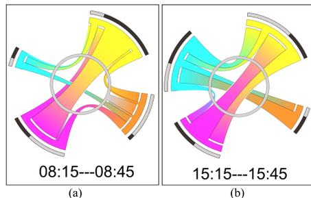
**Figure 10:** Comparison of lower (left) and higher (right) ICU ratings at a road junction during different time periods. (a) The traffic flow from yellow to violet dominates the junction utilization; moreover, both the orange and yellow connecting links are highly unbalanced. (b) Traffic flows from different links in the junction are fairly balanced and the incoming/outgoing flows for each connecting links are also fairly balanced.
